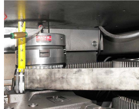
Photo 2: Clutch Operating with Overhung Load
