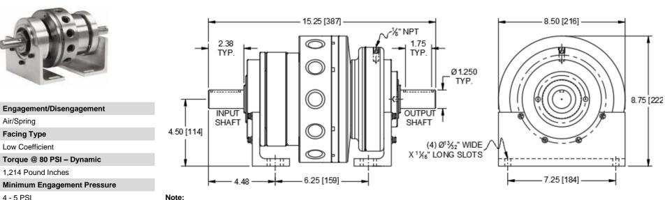
This clutch has a designated input and output shaft. Thermal-Horsepower ratings are only valid if the clutch is oriented in this manner.
