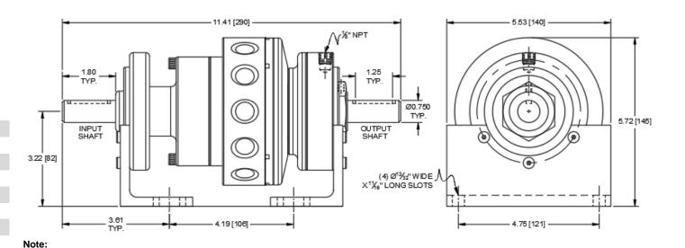
This clutch has a designated input and output shaft. Thermal-Horsepower ratings are only valid if the clutch is oriented in this manner.
