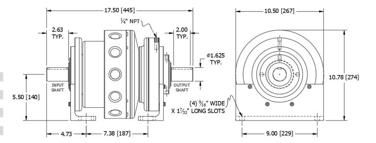
This clutch has a designated input and output shaft. Thermal-Horsepower ratings are only valid if the clutch is oriented in this manner.
