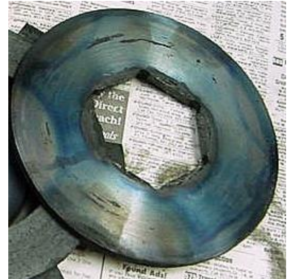
Heat Damaged Drive Disc of an Undersized Clutch
