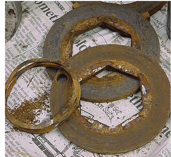
Drive Discs & Wave Spring Corroded By Moisture
