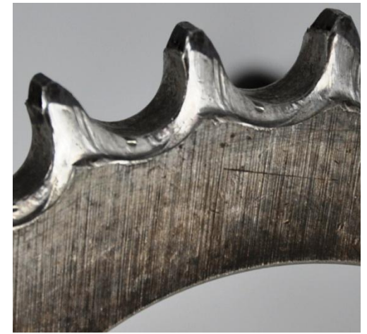
Sprocket Worn from Misalignment
