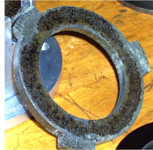
Friction Disc Contaminated With Brake Cleaner
