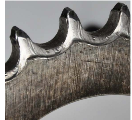
Photo 3: Sprocket Worn from Misalignment
